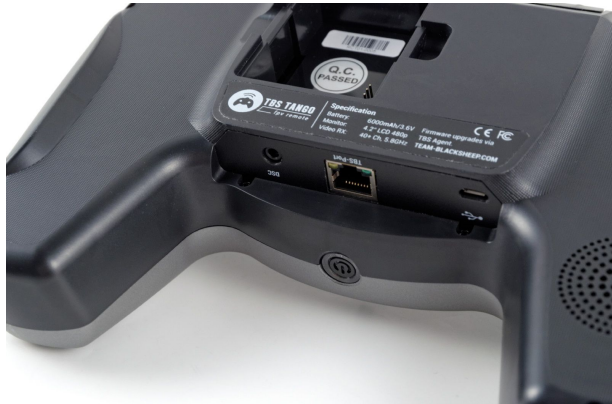
JR-module slot, DSC, micro-USB, TBS-port (for goggles), power button and speaker
