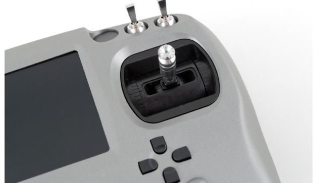
Right gimbal for aileron and elevator, and digital pad for trims
