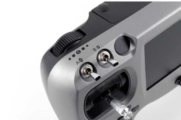
Three-position (A/L2), two-position (B/L1) switch, spring-loaded dial (SW E) and video receiver bay
